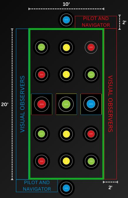
This setup is designed for head-to-head competition but can also be run with a single team at a time. In that case, only one side of the flight zone is needed, and seven landing pads will be required.
